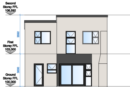
TYPICAL REAR ELEVATION Scale 1:100
