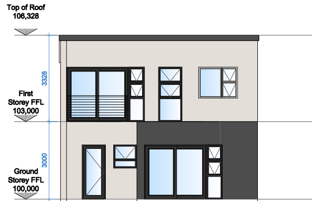
TYPICAL REAR ELEVATION Scale 1:100
