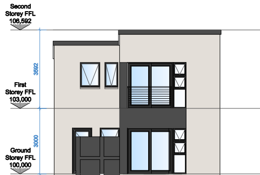
TYPICAL REAR ELEVATION Scale 1:100
